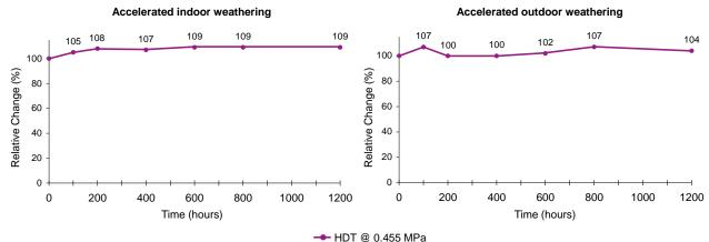
Note: For the indoor method, it is possible to infer that accelerated weathering times of 400 and 800 hours correspond to ca. 5 and 10 years of ageing in normal conditions, respectively. For the outdoor method, it is possible to infer that accelerated weathering times of 400 and 800 hours correspond to ca. 8 and 16 months of ageing in normal conditions, respectively.
